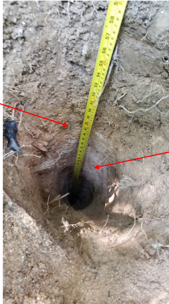
Plate 10 Open hillslope colluvium revealed at IP5 (about +136 mPD) near the lower portion of the NTSA
