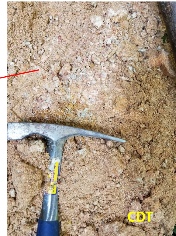
Plate 10 Open hillslope colluvium revealed at IP5 (about +136 mPD) near the lower portion of the NTSA
