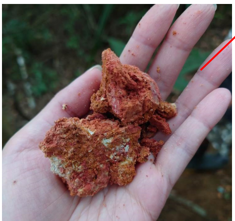
Plate 7 Open hillslop colluvium revealed at IP2 (about +183 mPD) in the vicinity of the upper portion of the NTSA
