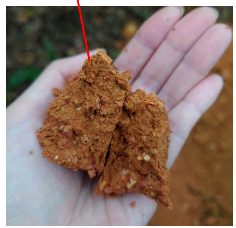
Plate 7 Open hillslop colluvium revealed at IP2 (about +183 mPD) in the vicinity of the upper portion of the NTSA
